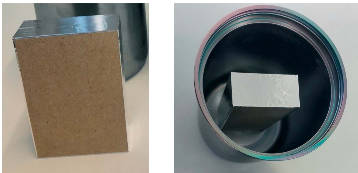
Figure 4. Medium-density fiber board (MDF) prepared in 6 cm x 9 cm size and all edges covered with aluminum foil. The sample was placed vertically in the DHS Large container.
