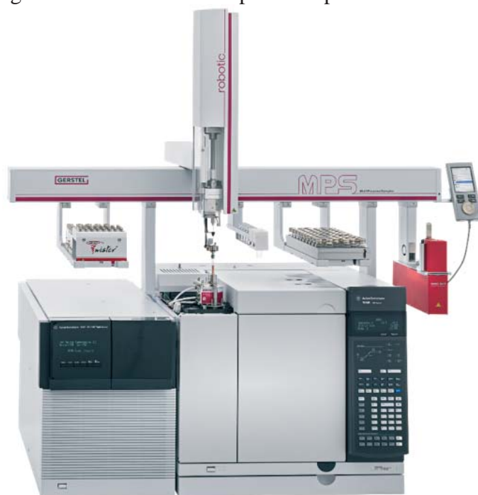
Figure 3. Automated DHS/ DHS large-TD-GC/MS system used in this work.
