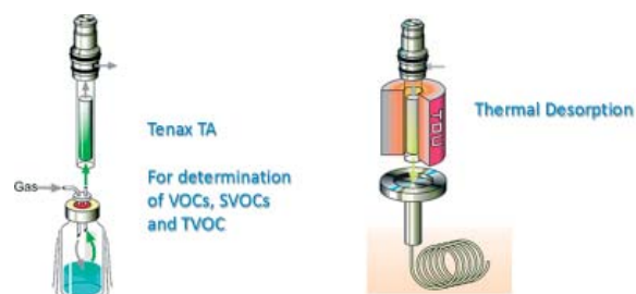
Figure 8. Tenax TA/TD-GC/MS method for the determination of VOCs, SVOCs and TVOC.
