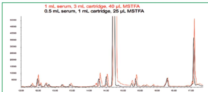
Analysis of THC and metabolites from serum with automated sample preparation. Extraction of 0.5 mL serum with 1 mL 100 mg C18ec SPE cartridge and 1 mL serum with 3 mL 200 mg C18ec cartridge. Reconstitution in 25 µL MSTFA or 40µL MSTFA respectively. Same performance is achieved, but the 1 mL cartridge requires less sample, less solvent, less elution volume, less time for evaporation, less MSTFA volume, less time for reconstitution, and therefore results in higher throughput.
