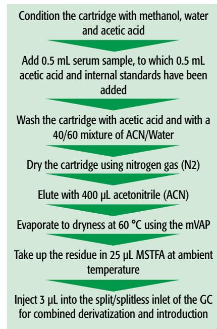
The separation was performed on a capillary column (VF-1 ms 25 m x 0.2 mm x 0.33 µm, Agilent Technologies) using a GC 6890 and MSD 5973 in single ion monitoring mode (SIM), both from Agilent Technologies.
