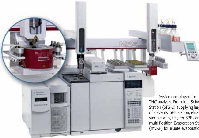
System employed for THC analysis. From left: Solvent Filling Station (SFS 2) supplying large volumes of solvents, SPE station, eluate and sample vials, tray for SPE cartridges, multi Position Evaporation Station (mVAP) for eluate evaporation
