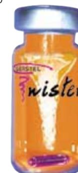
bar spins in the sample, organic compounds are extracted into its polydimethylsiloxane (PDMS) coating. The Twister can be used with matrices as diverse as drinking or wastewater, body fluids, beverages, dairy products, and processed foods. After sample extraction, the Twister can be directly transferred to the GERSTEL TDS 2 thermal desorption system where the extracted compounds are thermally desorbed and determined by gas chromatography. For a more detailed look at Twister, see pages 4 – 8.
