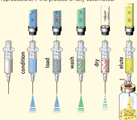
1. Standard 1, 3 or 6 mL SPE cartridges are available equipped with transport adapters for easiest possible automation using the GERSTEL SPE. An added benefit is that the GERSTEL SPE cartridges have practically no dead volume.
