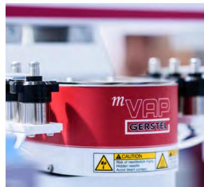
GERSTEL Multi-Position Evaporation Station ("mVAP")
