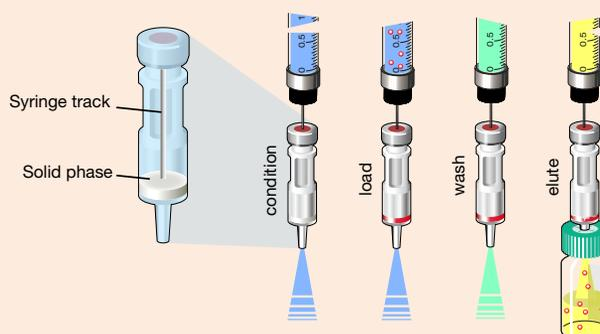
After conditioning the sorbent, the cartridge is loaded with sample. If necessary, the sorbent bed can be washed to remove matrix components before elution is carried out in the final step using a suitable solvent. Compared to conventional SPE, this process requires significantly less solvent due to the lower quantity of sorbent (10 - 45 mg).
