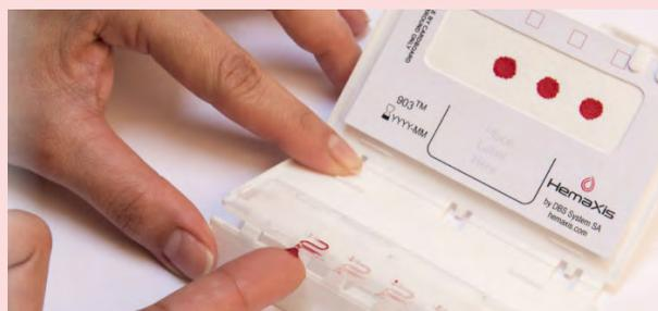
Simple and exact sampling of a 10  $\mu$ L volume of whole blood onto Dried Blood Spot (DBS) cards. Image: DBS System
