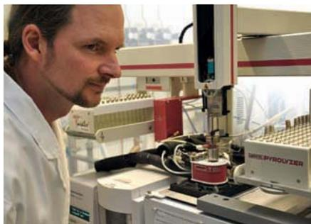
existing GC/MS hardware and software. The idea behind the project is to enable automation of the established GERSTEL pyrolysis technology based on the company's MultiPurpose Sampler (MPS), adding pyrolysis to a long list of automated sample preparation and introduction techniques for GC/MS.
