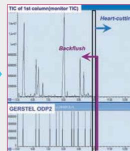
Simultaneous MS and olfactory detection is possible in both 1D and 2D GC analysis modes.
