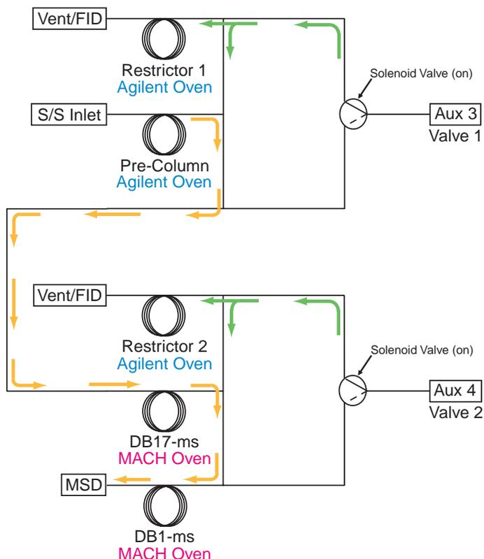
**Figure 2.** Flow diagram of dual Dean's switch.
