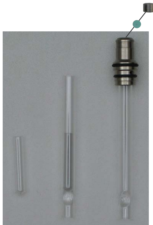
Figure 2. Microvial, GERSTEL TDU-liner and septum top.
