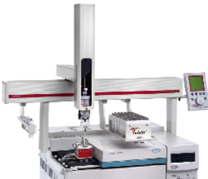
Figure 1. GERSTEL MPS 2 with TDU and ATEX option mounted on an Agilent 6890 GC.
