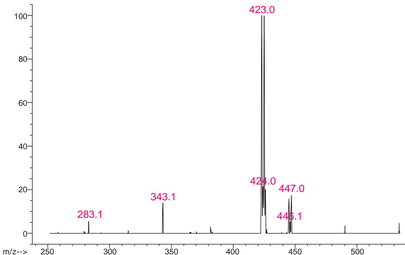
**Figure 4.** Mass spectrum of monobrominated aflatoxin B1.
