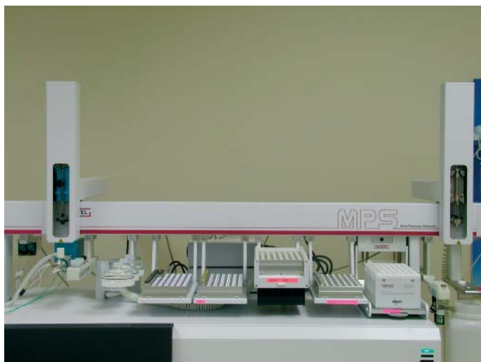
Figure 1. MultiPurpose Sampler (MPS XL) with GERSTEL DPX Option used for the automated hydrolysis and DPX-LC/MS/MS method.
