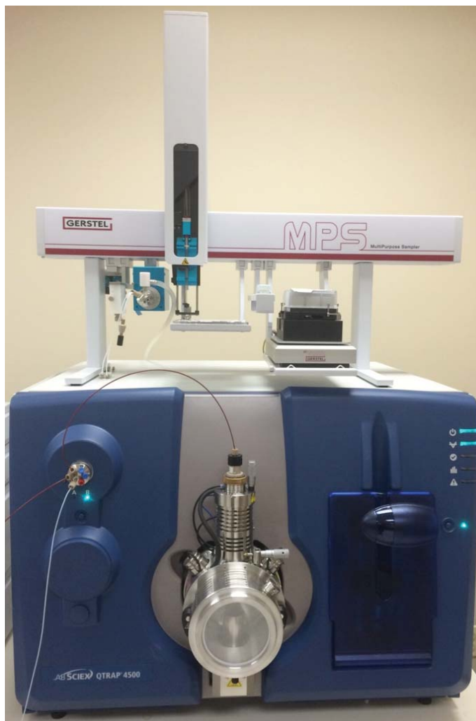
Figure 1. GERSTEL MultiPurpose Sampler (MPS) configured with an AB SCIEX QTRAP® 4500 LC/MS/MS system.
