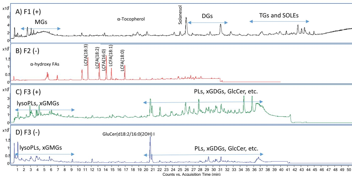
**Figure 4.** Total ion chromatograms of LC-QTOF analyses of the SPE fractions. A: fraction 1 in ESI POS mode, B: fraction 2 in ESI NEG mode, C: fraction 3 in ESI POS mode, D: fraction 3 in ESI NEG mode.
