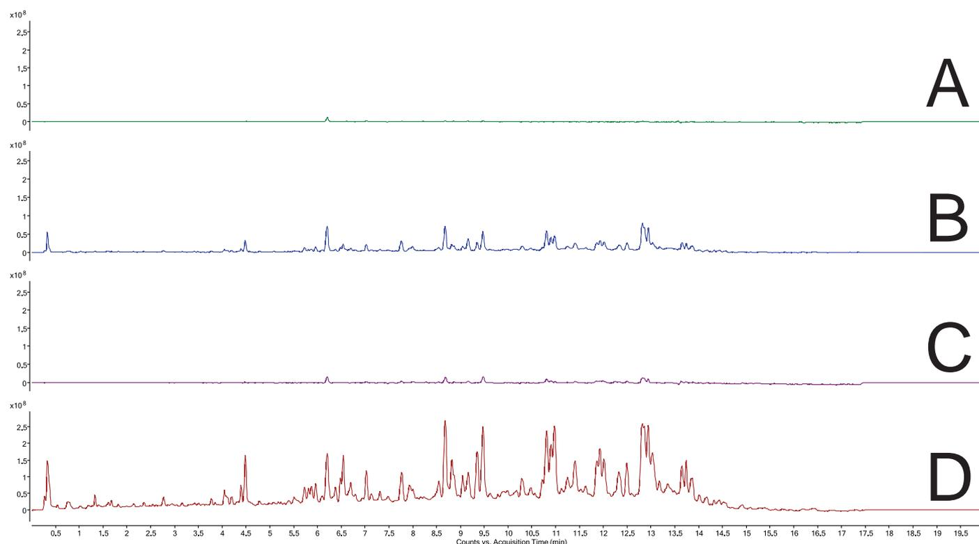
**Figure 5.** Comparison of background matrix interference between increased volumes of QuEChERS extracts for ground organic ginger, combined with dSPE and SBSE cleanup respectively. A: 1 mL with SBSE, B: 1 mL with dSPE, C: 7.5 mL with SBSE, D: 7.5 mL with dSPE.
