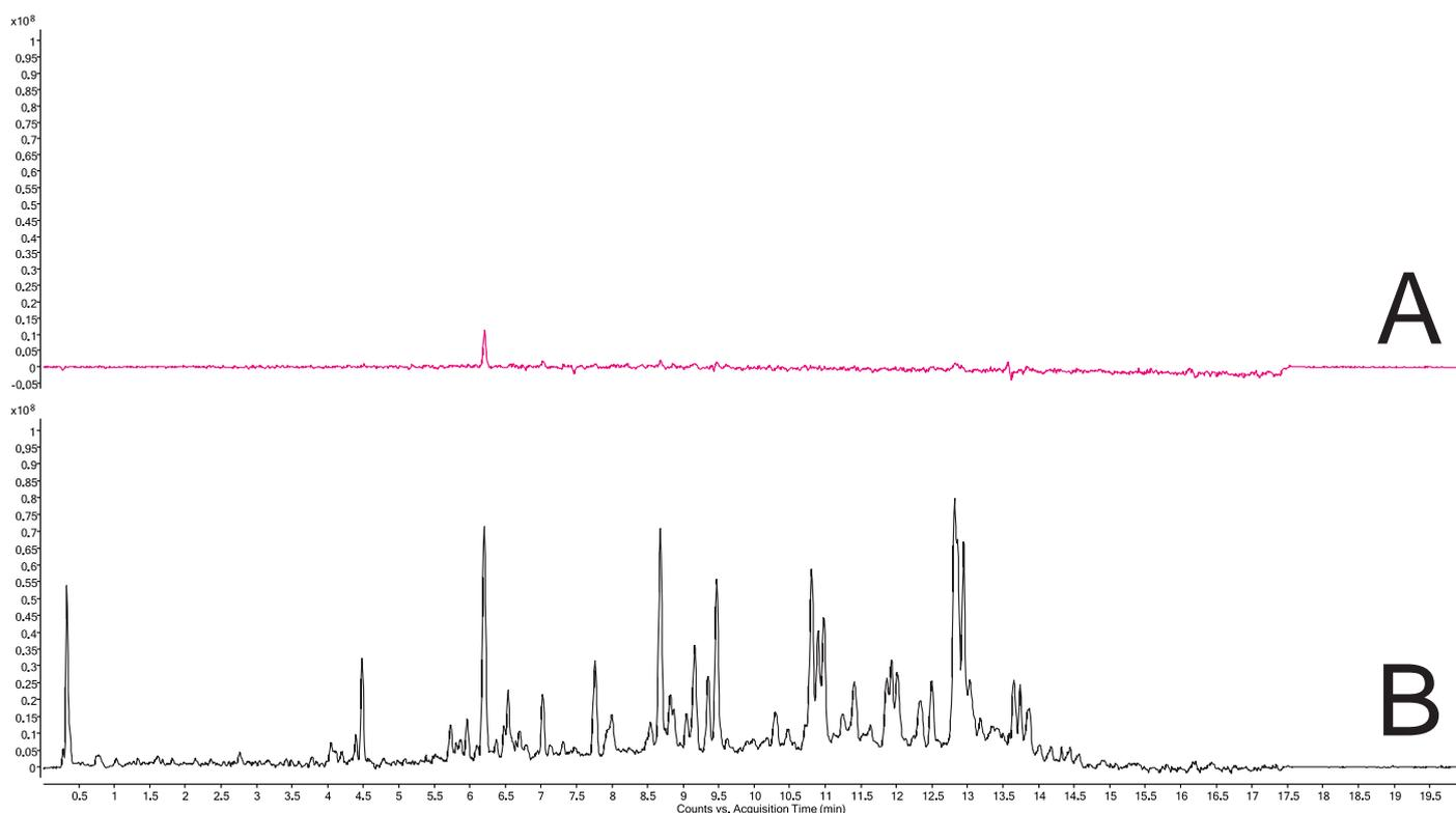
**Figure 4.** Comparison of background matrix interference between 1 mL of 1st QuEChERS extract combined with SBSE (A) and 1 mL of 1st QuEChERS extract combined with dSPE (B) for ground organic ginger.
