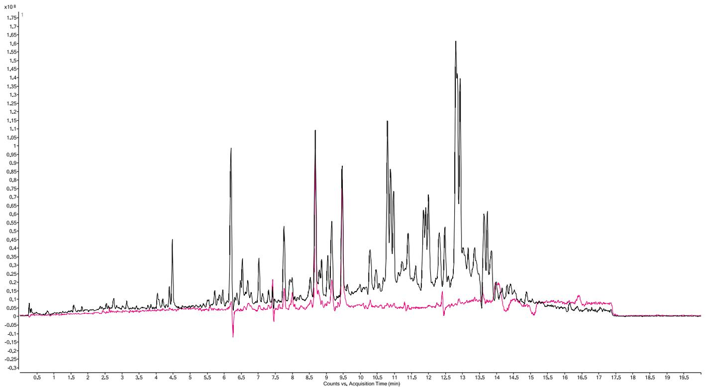
**Figure 2.** Comparison of background matrix interference between QuEChERS (black trace) and QuEChERS combined with SBSE (red trace) for ground organic ginger. Full scan ( $m/z$  85-550) Frag 135; blank mobile phase subtracted from each TIC.
