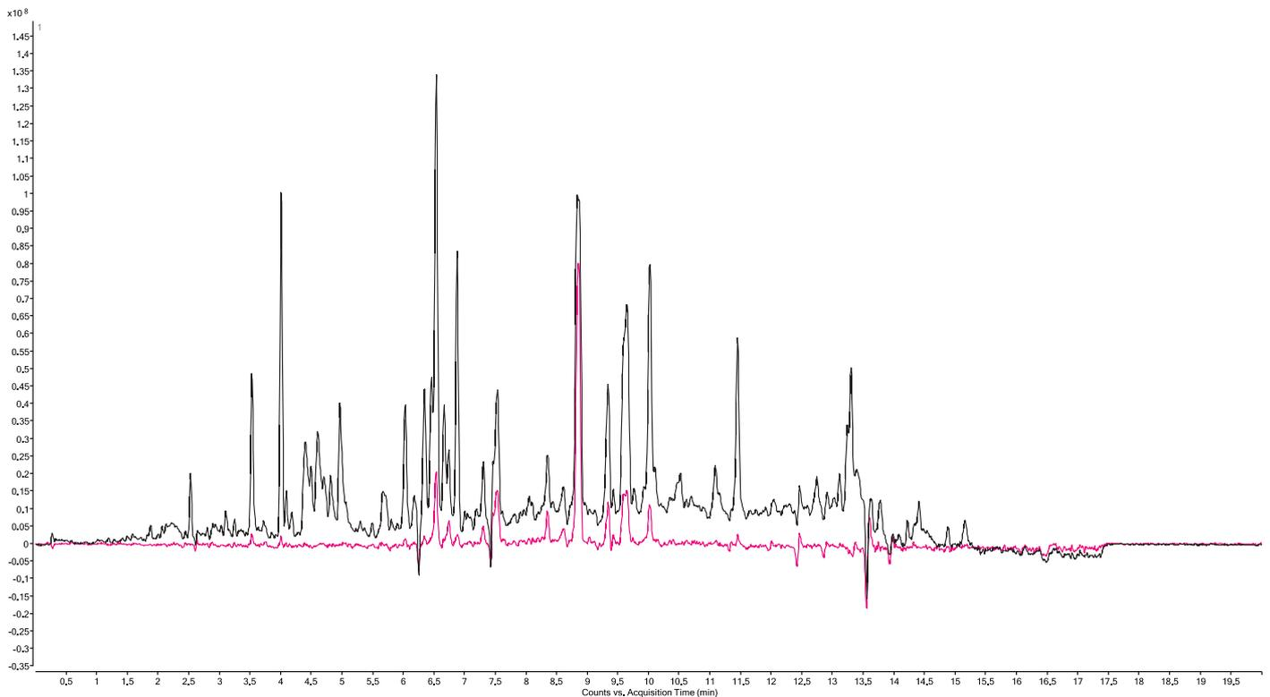
**Figure 3.** Comparison of background matrix interference between QuEChERS (black trace) and QuEChERS combined with SBSE (red trace) for ground organic turmeric. Full scan ( $m/z$  85-550) Frag 135; blank mobile phase subtracted from each TIC.
